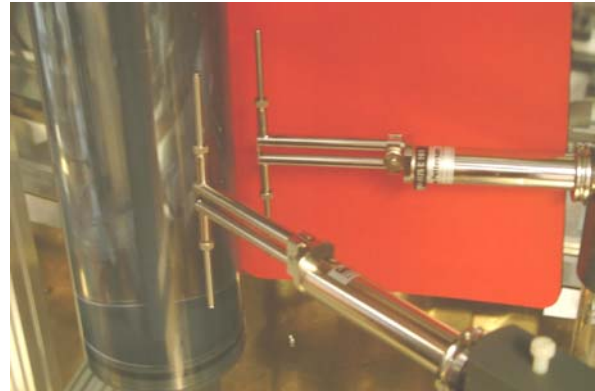
Figure 2. Two parallel dipoles 2 cm from lossy cylinder.
